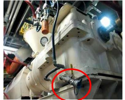
Quick-connect on gearbox for filter cart
