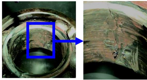
Fretting can occur on the inner ring of bearings where they meet the shaft
